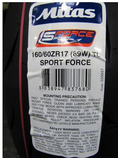
During sustained high speed riding a bulge may appear on the tread of the tyre causing vibration and in the most extreme of cases some of the tread may become detached. This problem has only been simulated in controlled and the most severe of conditions. The Sport Force recall is pre-emptive.
